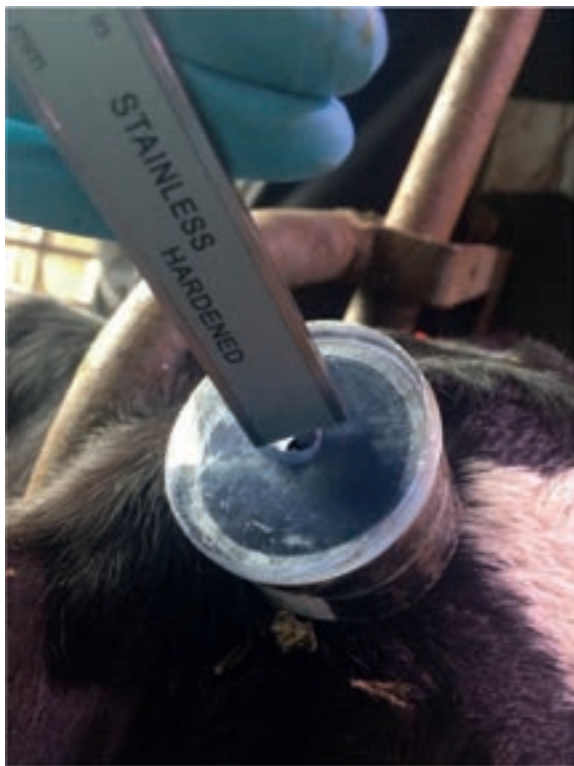
Fig. 1 Methodology used to measure horn bud height showing the depth gauge of the calliper (model 49–923-150; Linear Tools, UK) positioned through the aperture of the cylinder (diameter 43 mm; height 30.85 mm) when placed over the horn bud
