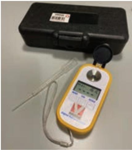
**Figure 1: Digital refractometer.**
