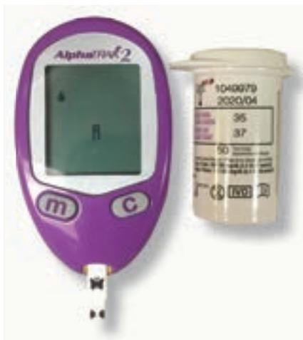
**Figure 4: Alphatrak 2 glucometer.**
